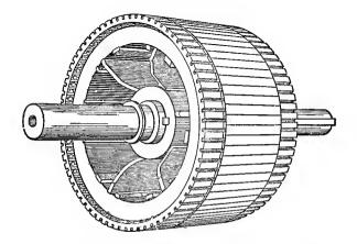
FIG. 138. Secondary core and conductors of a. c. induction motor.
